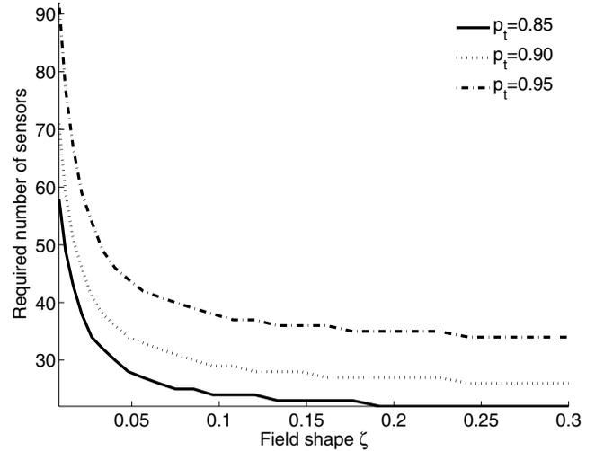
Fig. 4. Effect of field shape parameter  $\zeta = D_1/D_2$  on the required number of sensors where total area is  $3000 \text{ m}^2$ ,  $d_t = 10$  m. and  $P_t = 0.85, 0.90, 0.95$ .
