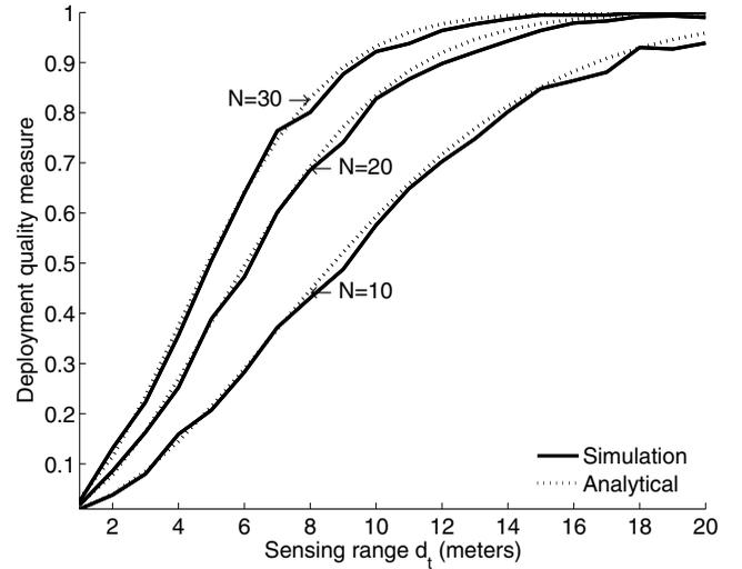
Fig. 1. Effect of sensing range on the DQM for  $D_1 = 30$  m,  $D_2 = 100$  m and  $N = 10, 20, 30$ .
