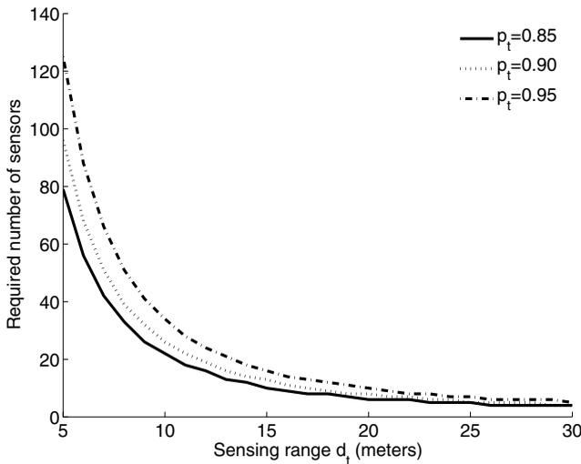
Fig. 3. Effect of sensing range on the required number of sensors for  $D_1 = 30$  m,  $D_2 = 100$  m and  $p_t = 0.85, 0.90, 0.95$ .
