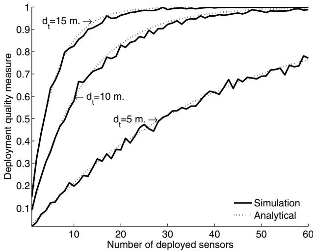
Fig. 2. Effect of number of sensors on the DQM for  $D_1 = 30$  m,  $D_2 = 100$  m and  $d_t = 5, 10, 15$  m.
