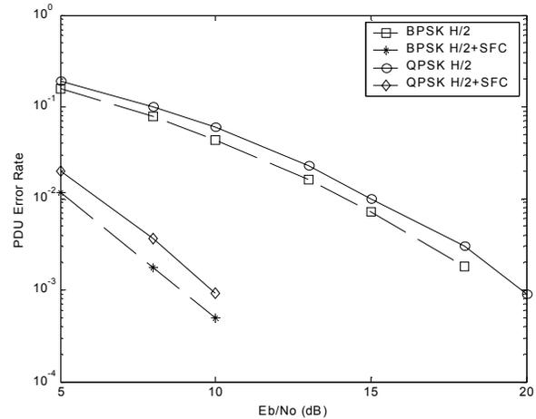
**Fig. 3. Simulation results of PDU error rates for BPSK and QPSK, averaged over 40 channels without SFC, and over 20 channel pairs with SFC (HIPERLAN/2 channel A).**
