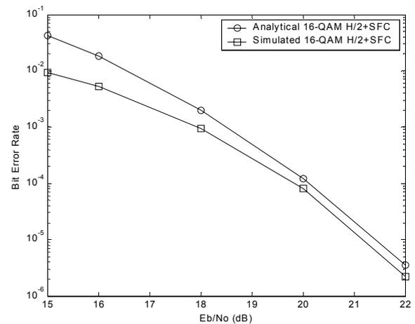
Fig. 8. Bit error rates for analytical and simulated 16-QAM with SFC.
