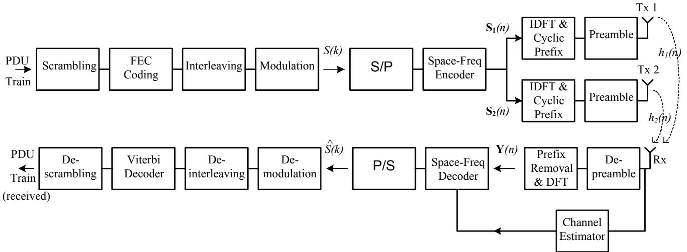
Fig. 2. Block diagram of HIPERLAN/2 with space-frequency coded double-transmit antenna diversity. In the figure,  $S_1(n)$  and  $S_2(n)$  are the  $n$ th coded OFDM blocks, and  $Y(n)$  is the corresponding received OFDM block.
