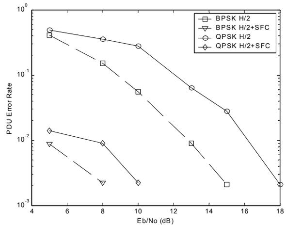
**Fig. 4. Simulation results of PDU error rates for BPSK and QPSK, with and without SFC through channels (25) and (26) (HIPERLAN/2 channel A).**
