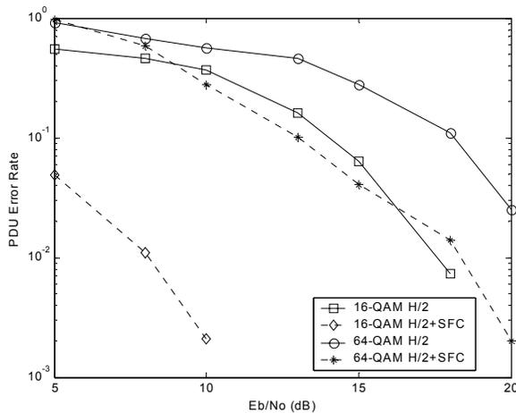
Fig. 6. Simulation results of PDU error rates for 16-QAM and 64-QAM, with and without SFC through channels (25) and (26) (HIPERLAN/2 channel A).
