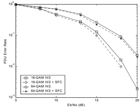
**Fig. 5. Simulation results of PDU error rates for 16-QAM and 64-QAM, averaged over 40 channels without SFC, and over 20 channel pairs with SFC (HIPERLAN/2 channel A).**
