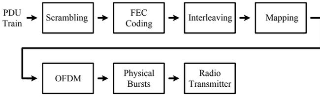
Fig. 1. The transmitter structure in HIPERLAN/2 [4].
