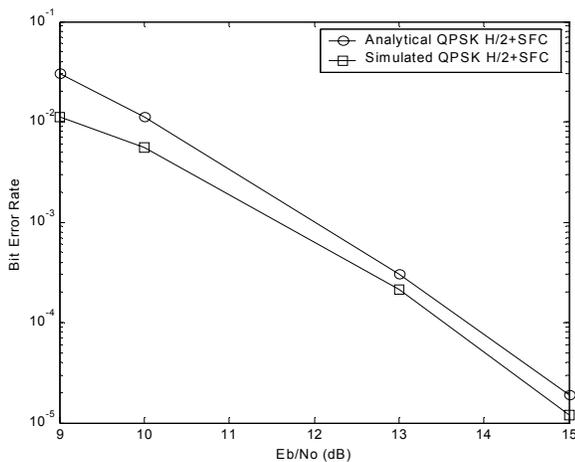
Fig. 7. Bit error rates for analytical and simulated QPSK with SFC.
